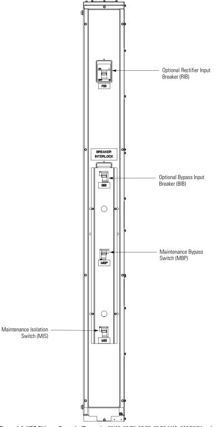
Figure 4-6. UPS Sidecar Controls (Bypass) – 80/40, 80/50, 80/60, 80/80 kVA, 208/208V and 160/100, 160/120, and 160/160 kVA, 480/480V with Optional BIB and RIB
